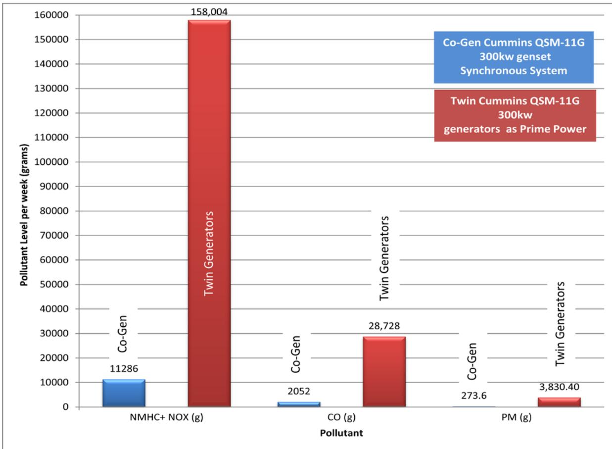
Figure 3 above shows a comparison of tailpipe emissions between a co-gen system (blue) and twin generators (red) comparably sized. Note the disparity in emissions levels when used under the same load conditions. A co-gen system uses the Grid power as the primary power source and only brings a generator on line when redundant power is needed whereas the twin generators must run 24/7
